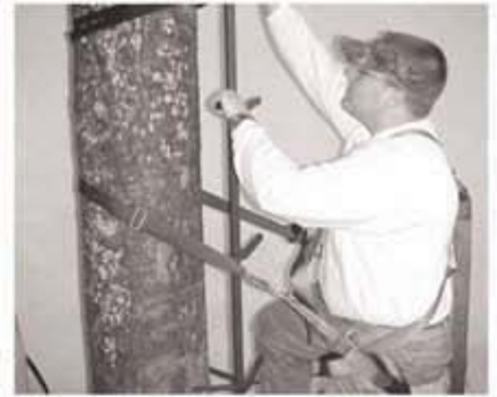
Figure 7- Adjust the Length as Needed for Hands Free Attachment
