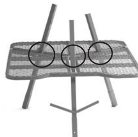
FIGURE 9 INSTALL UPPER PLAT- FORM SUPPORTS AND LADDER
