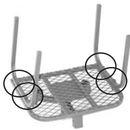
FIGURE 4 INSTALL U-BRACES ON STANDING PLATFORM
