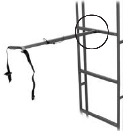
FIGURE 21 INSTALL TREE STABILIZER BAR
