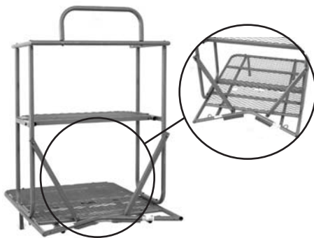
FIGURE 10 INSTALL REAR DIAGONAL BRACES
